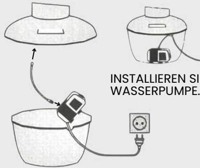
INSTALLIEREN SIE DIE WASSERPUMPE.
